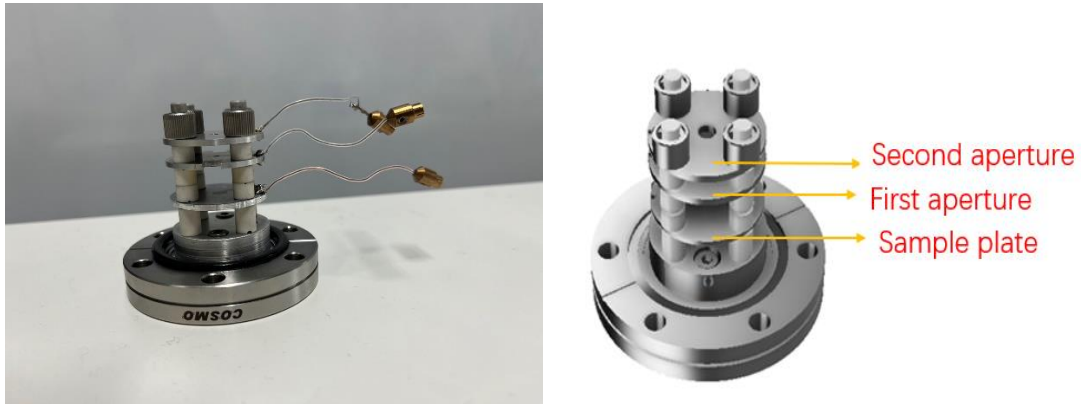
Figure 2.10 - Picture of two-stage acceleration electrodes (left) and 3D CAD drawing (right)
